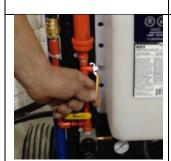
7. Press briefly the RED button on the dosage selector to charge the air treatment fluid in the INJECT-AIR.  $\ast\ast$
