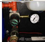
3. Connect the INJECT-AIR's pressure entry port to the shop's air supply with a hose and adjust the pressure regulator to desired pressure (do not exceed 130 PSI). \*
