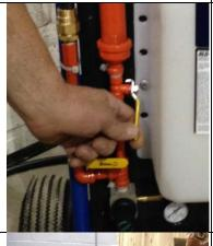
15. Slowly open the INJECT-AIR's air control valve and charge service control line until vapor / liquid exhaust from the trailer's supply line and shut the INJECT-AIR's air control valve.
