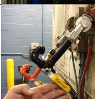
16. Connect the air supply delivery port (black) to the trailer's supply line.
